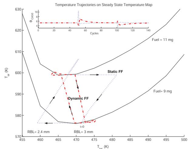
Fig. 8. Temperature trajectories and combustion timing with static and dynamic feedforward RBL controllers for fuel steps 9→11 mg/cycle and 11→9 mg/cycle.
