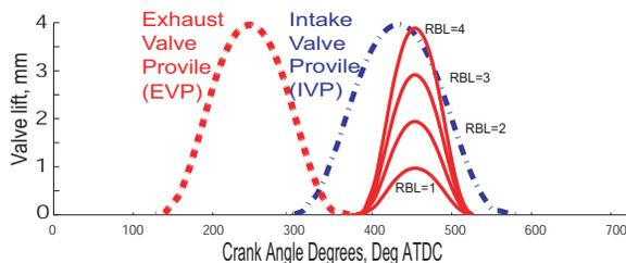
Fig. 1. Exhaust, intake and rebreathing valve profiles.
