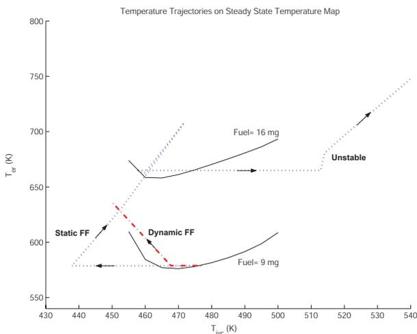
Fig. 9. Temperature trajectories with static and dynamic feedforward RBL controllers for fuel steps 9→16 mg/cycle and 16→9 mg/cycle.
