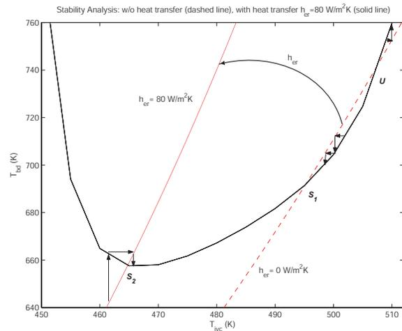
Fig. 6. Stability analysis through the recursive mapping between  $T_{ivc}$  and  $T_{bd}$  for fuel flow rate fixed at 9 mg/cycle.
