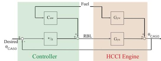
Fig. 7. Block diagram of the HCCI engine plant with a dynamic (cancellation) feedforward controller and an integral feedback controller.
