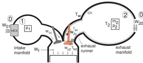
Fig. 2. Schematic diagram of the engine.
