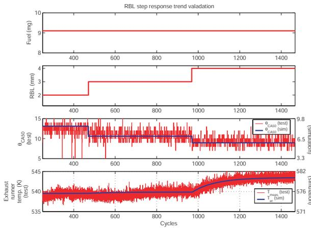
Fig. 4. Rebreathing lift step response trend validation.
