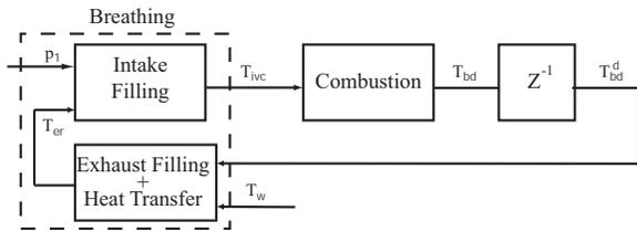
Fig. 3. The thermal feedback constituted by the breathing characteristics (including heat transfer in the exhaust runners and exhaust manifold) and the combustion characteristics of the HCCI engine with large percentage of residual gas in the cylinder charge.
