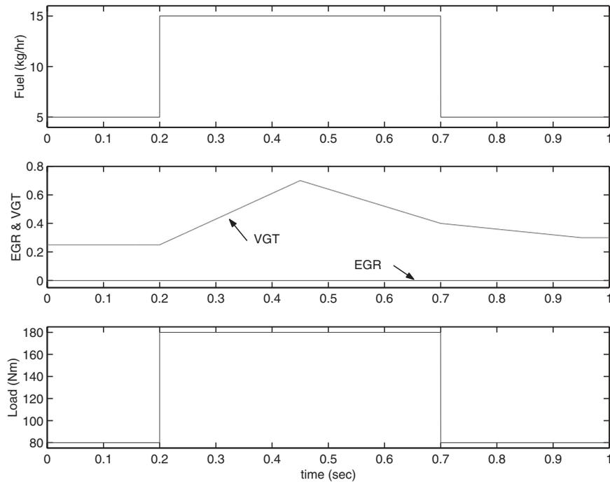
Figure 2. Inputs to the mean-value engine model.
