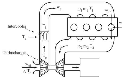
Figure 1. A turbocharged diesel engine with intercooler.
