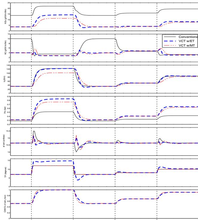
Figure 4: Comparison of the conventional, VCT w/ET, and VCT w/MT engines in response to a series of  $PP$  steps (12, 7, 8, 10 degrees) at 2000 RPM and cam risetime equal to 2 engine cycles. From top to bottom: NOx, HC, torque, manifold pressure, air-fuel ratio, throttle, and cam phasing.
