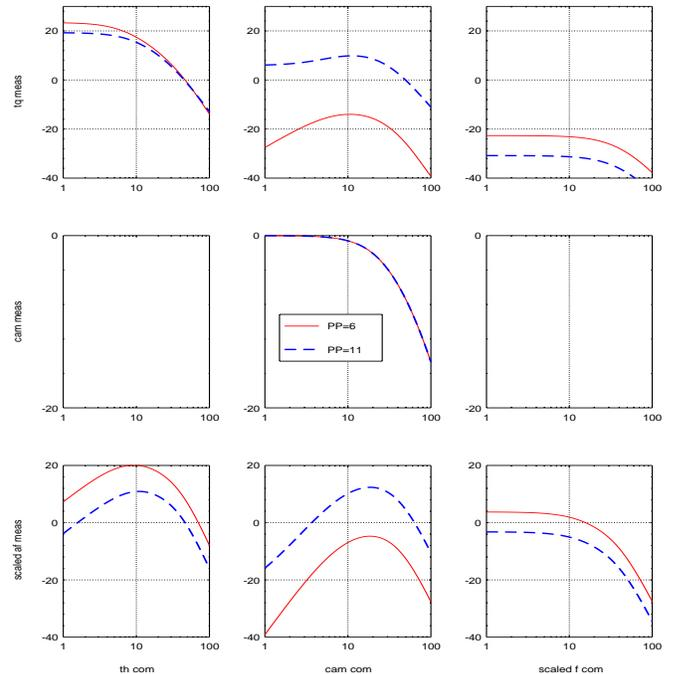
Figure 1: Open-loop Bode magnitude plots (in rad/sec) of the VCT engine at 2000 RPM linearized around PP=6 and PP=11 degrees. The nominal cam input is a function of pedal position to be described in Section 5.1., and the nominal fuel input is 0 g/intake stroke in both cases.
