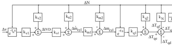
**Figure 4:** Linearized model of the camless unthrottled engine
