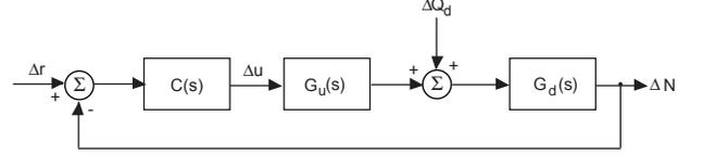
**Figure 5:** Unity feedback control system for the camless unthrottled engine.
