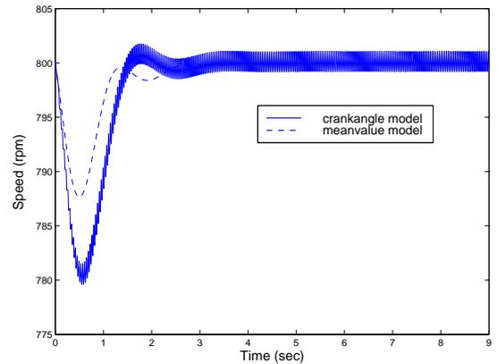
**Figure 6:** Step disturbance response for the closed loop mean-value and crankangle-based system.
