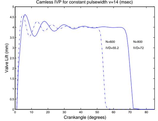
**Figure 3:** Intake valve profile for constant input pulsewidth ( $v = 14$  ms) for 800 and 600 rpm.
