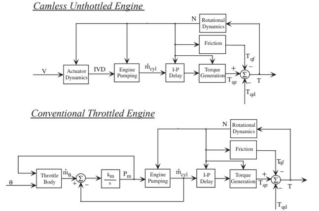
**Figure 1:** Nonlinear model of the camless unthrottled and the conventional throttled operation.
